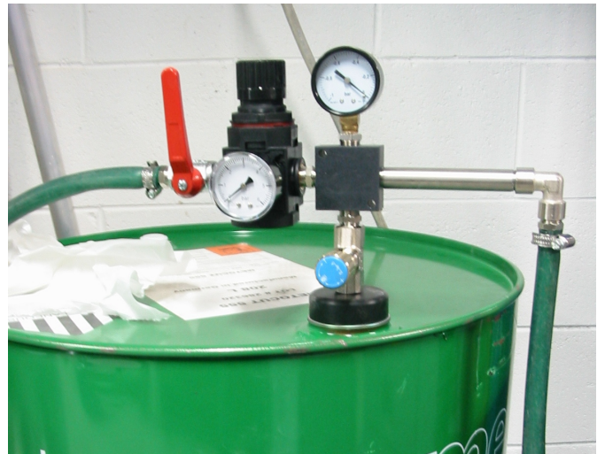
The water pressure gauge and the vacuum gauge, the latter if it indicates a value higher than 0.5/0.6 BAR the mixer is operating
