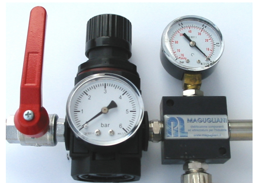
The water pressure gauge and the vacuum gauge, the latter if it indicates a value higher than 0.5/0.6 BAR the mixer is operating
